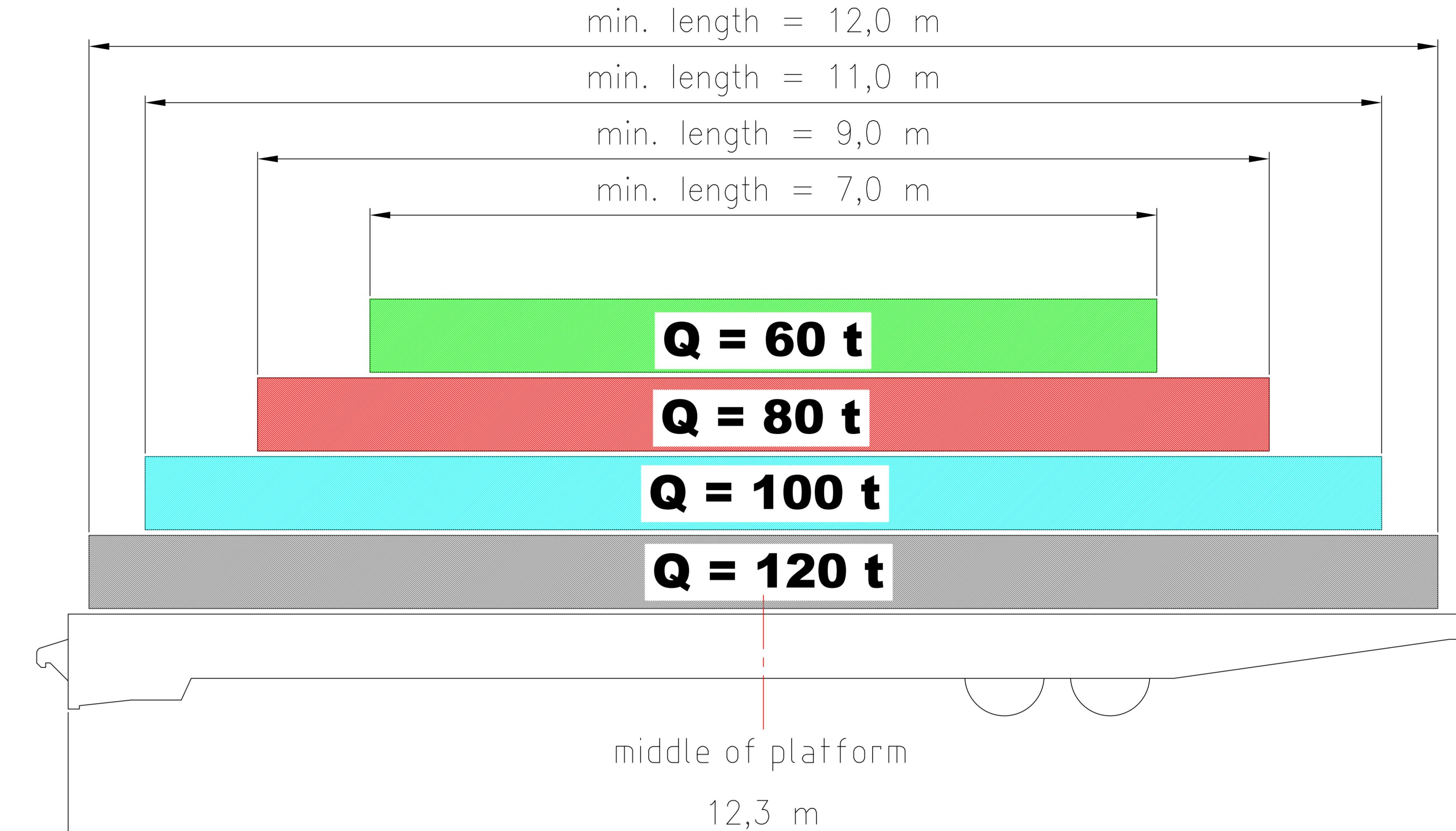
Load gravity center must be inside the respective marked areas
